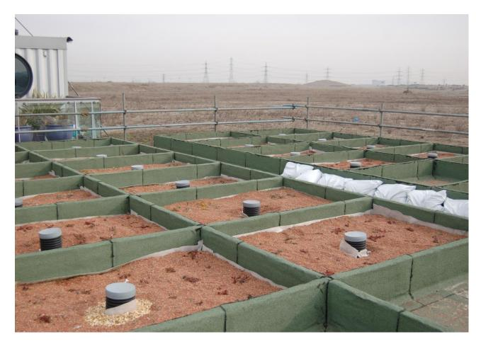
Figure 5. Installed green roof test bays at Barking Riverside Offices.
