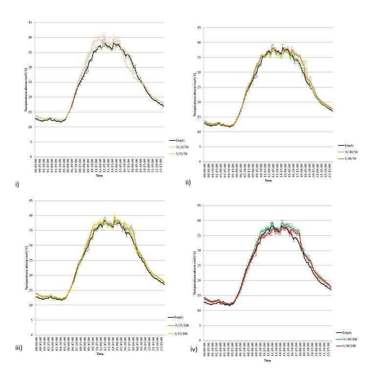
Figure 20. Average temperature immediately above the green and control roofs at Barking Riverside on one of the hottest day of 2013 (13th July) [Data for hottest day unavailable due to power cut on site]. i) Green roof pair W/25/50 and S/25/50; ii) Green roof pair W/40/50 and S/40/50; iii) Green roof pair W/25/100 and S/25/100; iv) Green roof pair W/40/100 and S/40/100. Error bars represent the standard error of the mean (n = 3).
