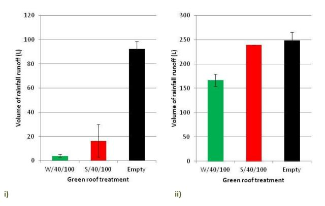
Figure 16. Average percentage rainfall attenuation for empty control roofs and 25 mm drainage, 100 mm substrate sedum and wildflower roofs at Barking Riverside for i) the summer months July to September 2010, and ii) the winter months October to December 2010. Error bars represent the standard error of the mean (n = 3).
