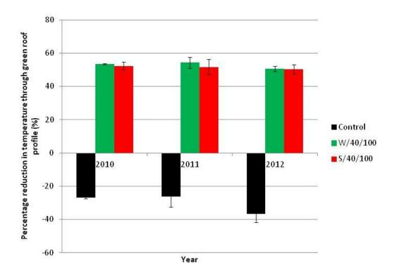
Figure 28. Average percentage reduction in temperature through control, W/40/100 and S/40/100 green roof profiles for the month of July, 2010 to 2012. Reduction in temperature calculated from the difference in temperature between sensor 4 (above the roof) and sensor 1 (beneath the roof). Error bars represent the standard error of the mean (n = 3).
