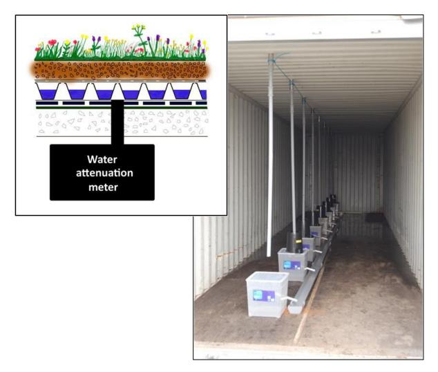
Figure 6. Plan and image of rainfall runoff monitoring equipment beneath the green roof test bays at Barking Riverside Offices.
