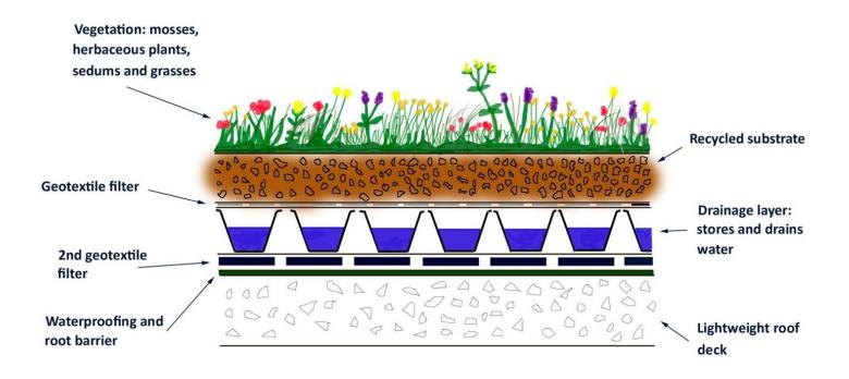
Figure 1. Typical extensive green roof design
