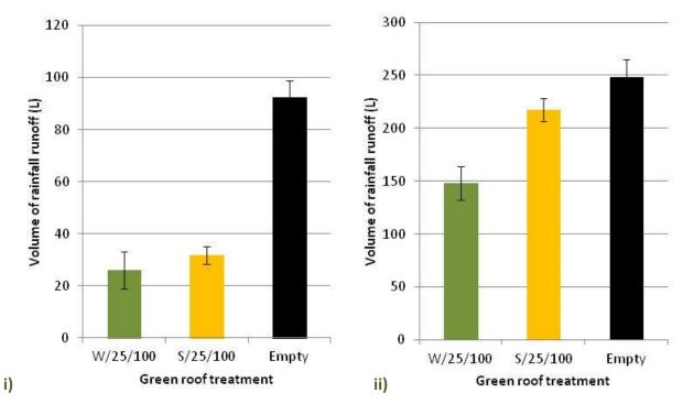
Figure 15. Average percentage rainfall attenuation for empty control roofs and 25 mm drainage, 100 mm substrate sedum and wildflower roofs at Barking Riverside for i) the summer months July to September 2010, and ii) the winter months October to December 2010. Error bars represent the standard error of the mean (n = 3).
