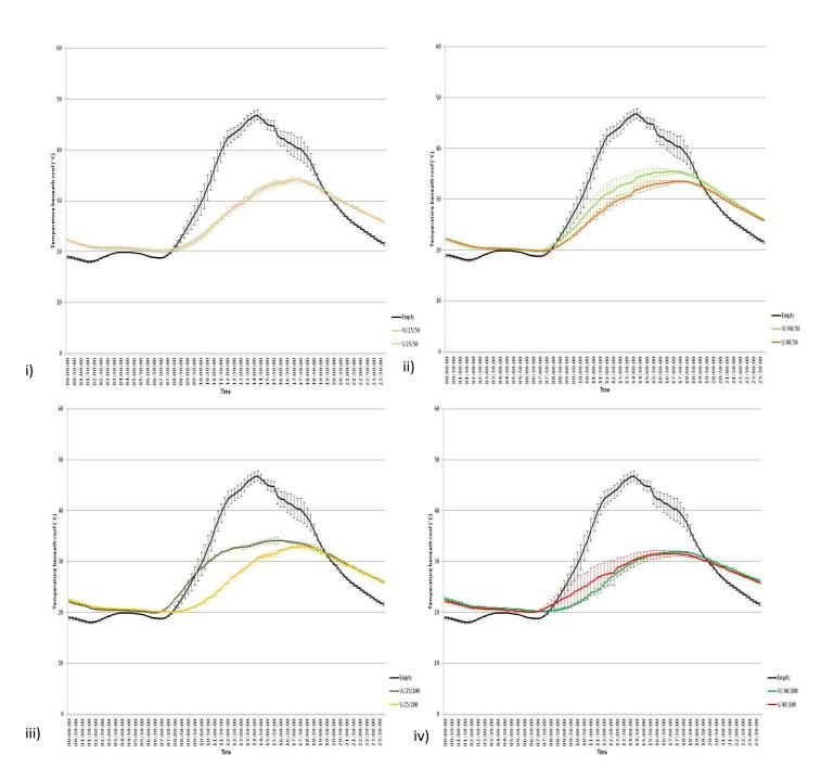
Figure 23. Average temperature immediately beneath each green and control roofs at Barking Riverside on the hottest day of 2012 (18th August). i) Green roof pair W/25/50 and S/25/50; ii) Green roof pair W/40/50 and S/40/50; iii) Green roof pair W/25/100 and S/25/100; iv) Green roof pair W/40/100 and S/40/100. Error bars represent the standard error of the mean (n = 3).
