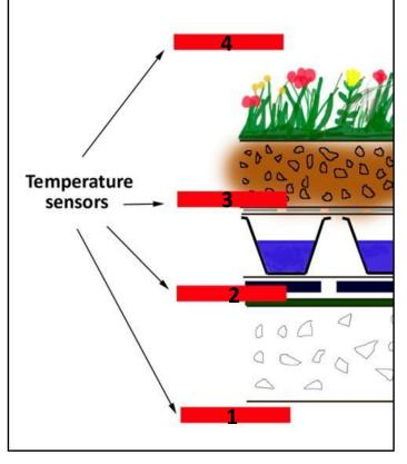
Figure 7. Plan of temperature senor monitoring equipment within the green roof test bay profiles at Barking Riverside Offices.
