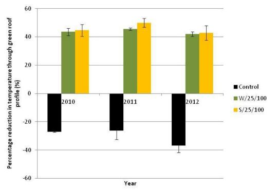
Figure 27. Average percentage reduction in temperature through control, W/25/100 and S/25/100 green roof profiles for the month of July, 2010 to 2012. Reduction in temperature calculated from the difference in temperature between sensor 4 (above the roof) and sensor 1 (beneath the roof). Error bars represent the standard error of the mean (n = 3).
