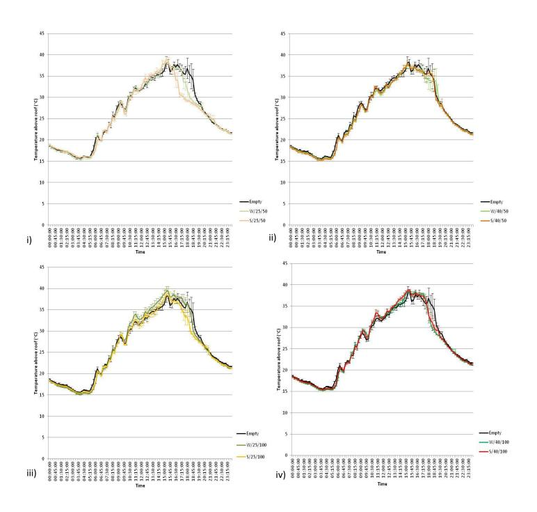
Figure 17. Average temperature immediately above the green and control roofs at Barking Riverside on the hottest day of 2010 (9th July). i) Green roof pair W/25/50 and S/25/50; ii) Green roof pair W/40/50 and S/40/50; iii) Green roof pair W/25/100 and S/25/100; iv) Green roof pair W/40/100 and S/40/100. Error bars represent the standard error of the mean (n = 3).
