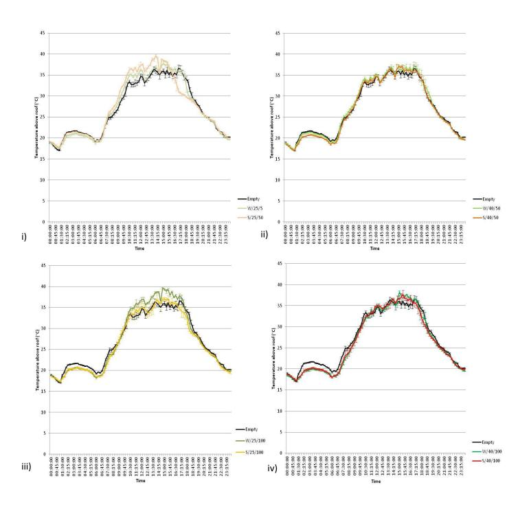
Figure 19. Average temperature immediately above the green and control roofs at Barking Riverside on the hottest day of 2012 (18th August). i) Green roof pair W/25/50 and S/25/50; ii) Green roof pair W/40/50 and S/40/50; iii) Green roof pair W/25/100 and S/25/100; iv) Green roof pair W/40/100 and S/40/100. Error bars represent the standard error of the mean (n = 3).
